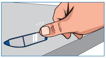
2 With your thumb located in the guard remover press downwards with your thumb and the guard will release with an audible click.
